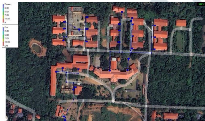
Fig 10: Pipe network for rainwater harvesting system- NSSCE
